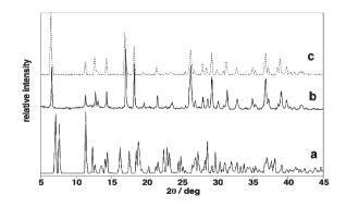
Fig. 3 (a) Calculated XRPD pattern of compound 1 before releasing the methanol molecule, (b) experimental XRPD pattern of 2, and (c) calculated XRPD pattern of  $\{Fe(3-CNpy)_2[Au(CN)_2]_2\} \cdot nH_2O$  ( $n \le 2/3$ ) (broken line) from ref. 7 data.
